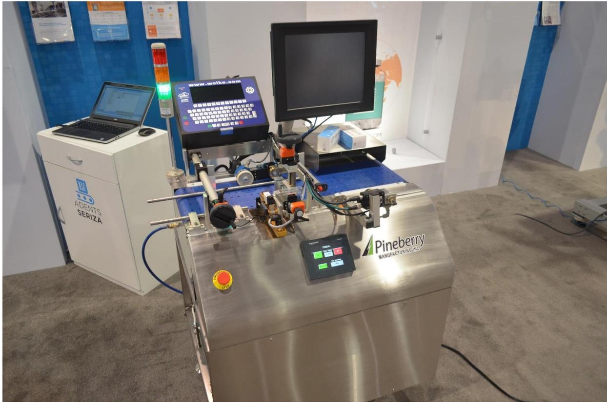
Erect cartons are coded and verified on the Pineberry CartonTrac EC erect carton packaging and serialization system, which can be installed as a standalone unit or integrated with other equipment.
