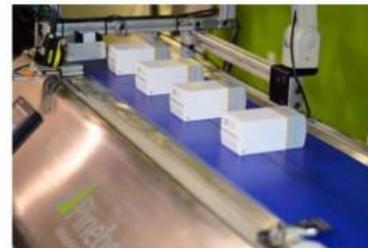
The CartonTrac EC erect carton packaging and serialization system consists of a vacuum conveyor, inkjet printer and camera system to apply and verify serialized codes.
