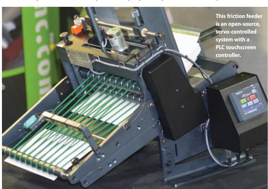
robustness, and cost efficiency. Also, they can be easily integrated into manual or automated lines. The HSF operates at 8,000 inches/min and the SF at 3,000.
