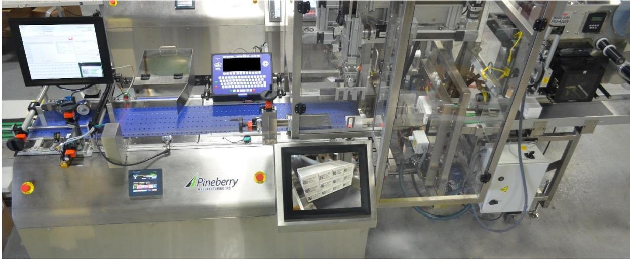
Pineberry CartonTrac serialization and aggregation system prints and verifies serialized codes on erect cartons and aggregates cartons in batches of 12.
