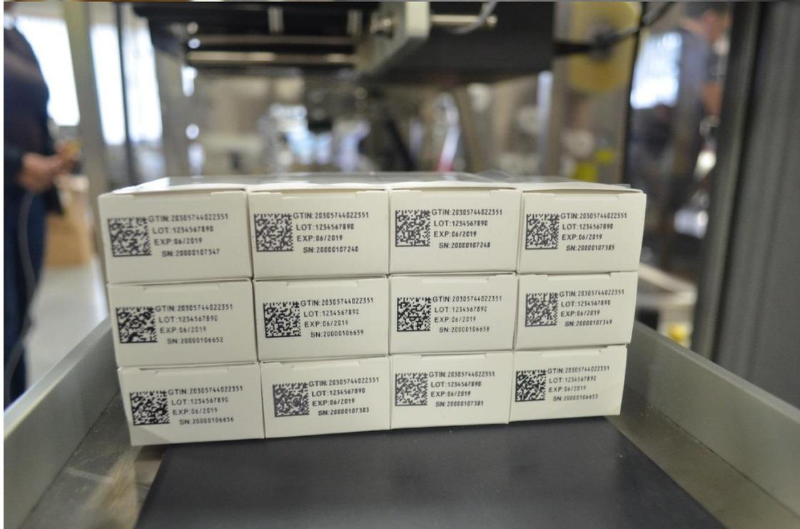
After exiting the CartonTrac system, aggregated bundles are loaded into master cartons, which are then palletized for shipment. Aggregated information is expanded at each step so scanning the pallet label will generate a list of each master carton, bundle and primary package in the load.
